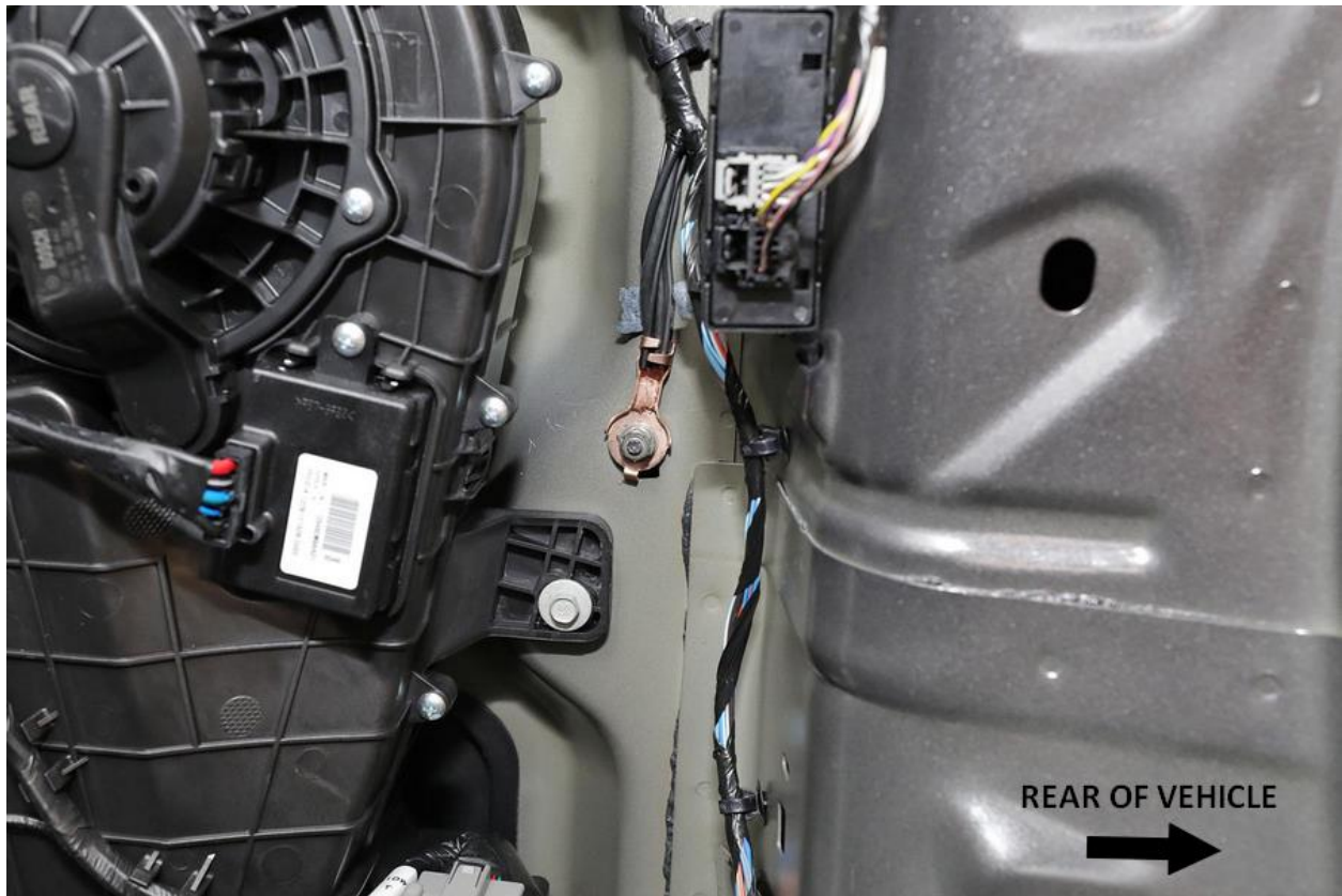
Figure 12: Passenger's Side D-Pillar Ground Location (Driver's Side Similar)
