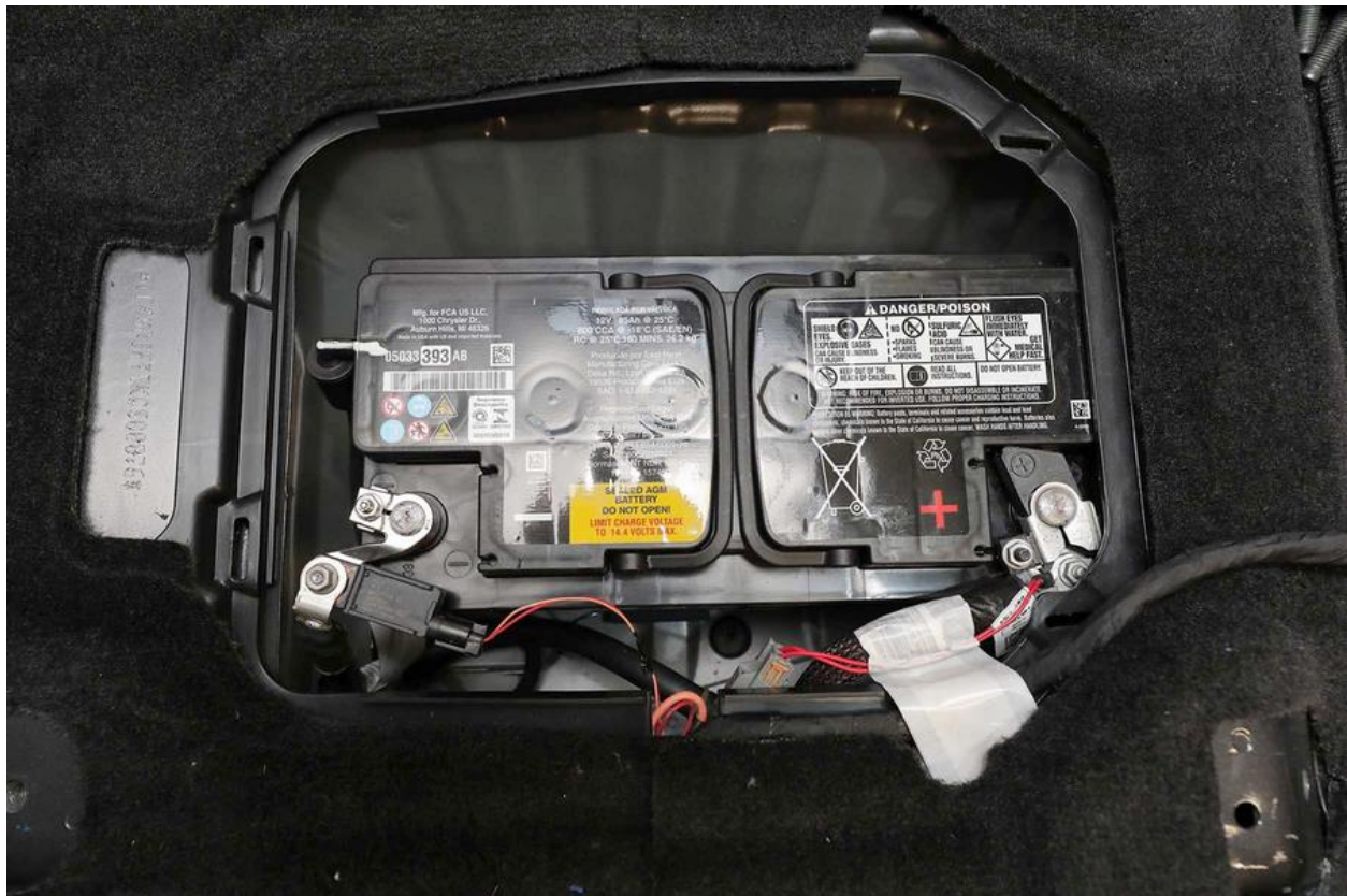
Figure 7: Battery Under Passenger Seat (V8 model shown)
