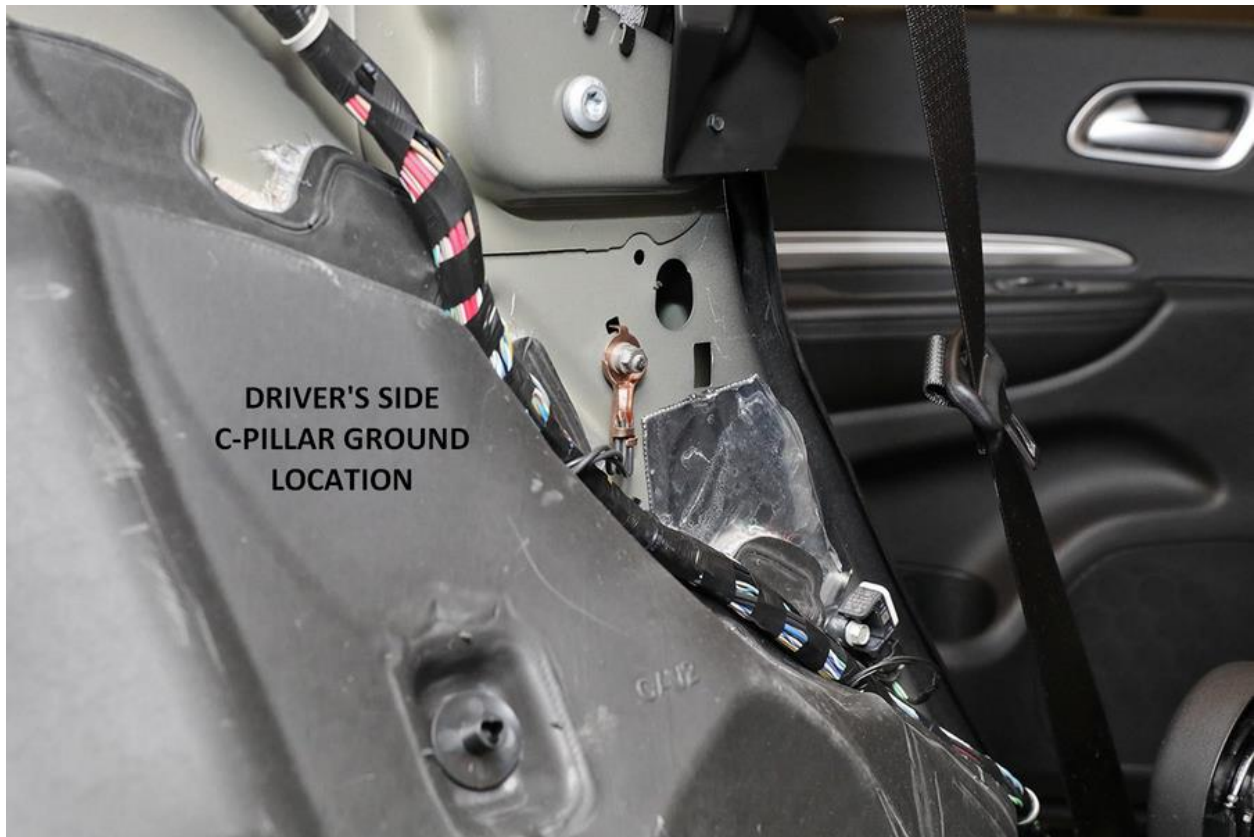
Figure 11: Driver's Side C-Pillar Ground Location (Passenger Side Similar)
